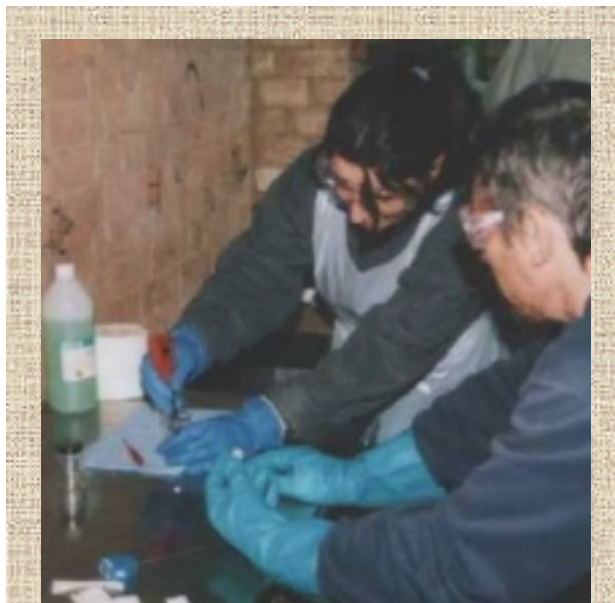
titration: Participants on a LILI 'How to Make Biodiesel' course carry out a titration test to calculate how much catalyst to use to make biodiesel from this batch of waste cooking oil
